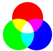
The default color mode for this controller is RGB666. Pixel colors are a combination of red, green, and blue color values. Each subcolor has 6 bits (64 different levels) of intensity. Equal amounts of red, green, and blue light produce white. Equal amounts of blue and green produce cyan. Red and green make yellow. Since each color component is specified by 6 bits, the final color value is 18 bits in length. The number of possible color combinations in RGB666 colorspace is 2^18 = 262,144 or 256K.
