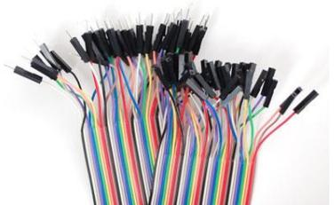
Male to female prototyping wires are very handy for making these point-to-point connections. Alternatively, you can bring out all of the GPIO lines to the breadboard with various third-party cables.
