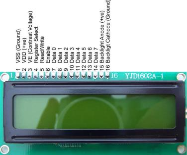
The LCD controller gives us two ways to send data: in one-byte (8 bit) chunks, or as two consecutive nibbles (4 bit). The second approach seems more complicated, but very frequently used. Why? It simplifies the hardware, and lets us talk to the LCD with half as many data lines. In general, I/O lines are a scarce resource! We use the 4-bit method on this board, and need only 6 I/O lines (2 control + 4 data) to communicate with the LCD.
