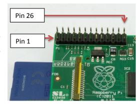
Here is a diagram of the pins and their functions. There are four pins for power and five pins for ground, leaving 17 pins for digital input/output. Of these, 9 (shown in blue) have alternative, specialized uses: 2 for I2C, 2 for UART, and 5 for SPI data communication. The remaining 8 lines in green are for general-purpose IO.
