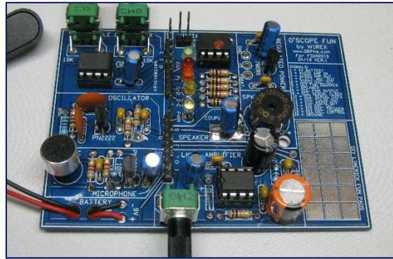
You just finished soldering-up your QRPme oscilloscope FUN board – now what? Where do you start? If you are like me, you plugged in a 9V battery and were relieved to see a few blinking LEDs. So far, so good. It is time to probe it with your oscilloscope.
