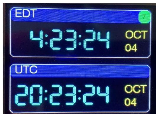
The final sketch for this series, **GPS\_CLOCK\_single**, adds 12/24hr display, local/UTC display. Touch control is used to toggle the options. (To enable touch, connect your display pins as follows: T\_DO to MISO, T\_DIN to MOSI, T\_CLK to SCK, and T\_CS to Blue Pill PA2. T\_IRQ remains unconnected. See my [touch tutorial](#) for more information.)
