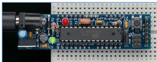
Instead of breadboarding an ATmega328 directly, I use the [DC boarduino](#) by Adafruit: it is breadboard friendly, and puts a DC power supply, microprocessor, external oscillator, ISP programming header, status LED, and reset switch all on a very small circuit board.
