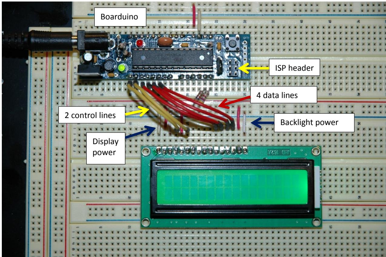
There are two control lines (yellow) and four data lines (red) between the PortB pins of the microcontroller and the display. The two resistors are for an I2C bus, not used in this demo.
