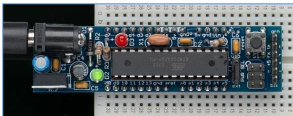
Next, you'll need a suitable 5V power supply for your breadboard. I started to wire up my micro, ISP-header, and power supply when I realized that I have a compact module containing all three: the [DC boarduino](#) by adafruit. This compact board contains the power supply, micro, and ISP header; plus a status LED and
