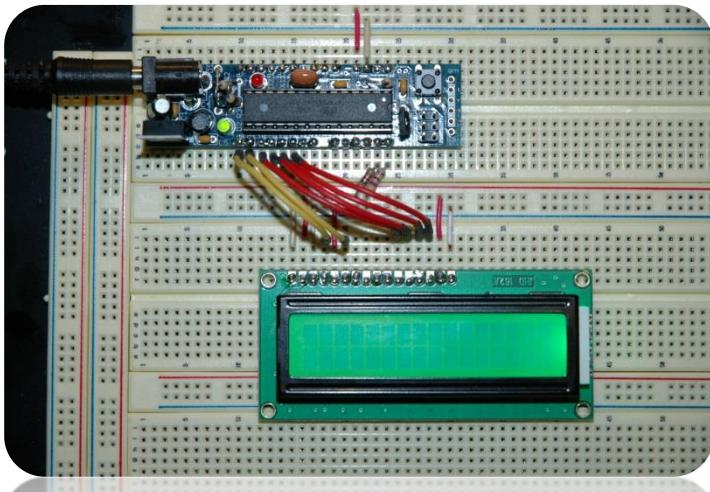
There are hundreds, if not *thousands*, of online articles about interfacing HD44780-compatible LCD displays to microprocessors/ microcontrollers. I have contributed one to the pile already, with my [write-up](#) on adding LCD displays to the Raspberry Pi. Here is what sets this article apart from the rest:
