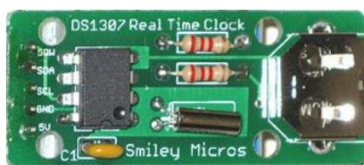
Next, you need a DS1307. Again I used a small circuit module rather than the chip. The module I used is the \$15 RTC kit by [Smiley Micros](#). The module adds the required external oscillator and battery backup. Other good ones are available from [SparkFun](#) and [Adafruit](#).
