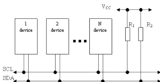
The interface circuit is “open collector”, which means that the data lines are passively kept high by resistors to Vcc. Any device on the bus can actively pull a data line low. Up to 128 devices can be put on the same data bus.
