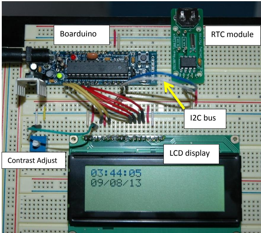
Here is the breadboard layout. The I<sup>2</sup>C bus is represented by the white (SDA) and blue (SCL) wires. There are two 4.7K pull-up resistors on the bus, which are partially hidden by the four red data lines. The LCD is a 20x4 character HD44780-compatible display. See my [LCD article](#) for more information on this interface. A 10K potentiometer controls the display contrast.
