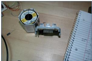
allows me to connect the keypad directly to a solderless breadboard for testing, or to a socketed rainbow ribbon cable I used for this project. Did you know that ribbon cable colors are in resistor color-code order?
