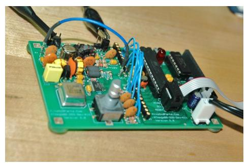
Notice that I don't even have my LCD connected! It doesn't do anything in the following experiments – in fact, we halt the microcontroller before the LCD is initialized. Looking at a nonfunctioning LCD was bothering me, so I removed it. Now find a group of lines, near the beginning of the program, that call SHIFT\_16 several times. The last group of 3 is listed here. Add a single instruction below it, like this:
