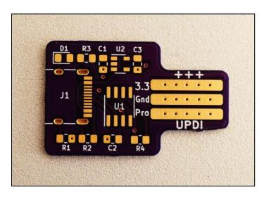
I chose to make mine from scratch. The result is a small dongle with three pogopins. To use it, press the pogo pins onto an unpopulated 3-pin PCB header (or machine pin socket). It's quick and easy, with no programming wires to connect and disconnect.
