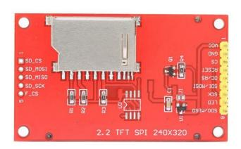
The interface is known as SPI (serial peripheral
