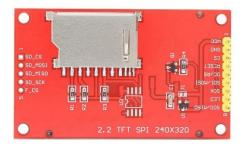
There are 5 pins on the display that connect to pins on the Blue Pill, and 3 pins that are power/ground related. The following table details the connections:
