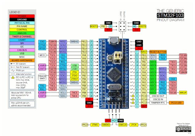
The Blue Pill has a full complement of digital and analog I/O pins; more than enough for this project.
