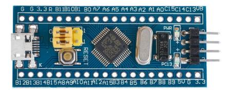
The microcontroller used in this project is the STM32F103C from ST Microelectronics. It is mounted on a very inexpensive board that is curiously named the "Blue Pill" (No, not <u>that blue pill</u>. This <u>blue pill</u>). Search eBay for suppliers and pick up a few. Current prices are \$2 to \$4 depending on shipping.
