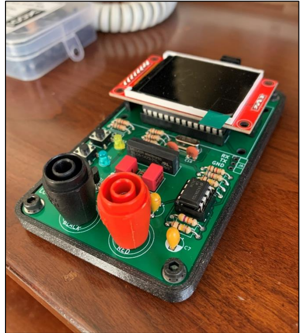
LC meter in a 3D-printed tray
