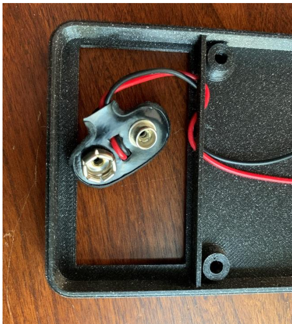
Securing the 9V battery clip
